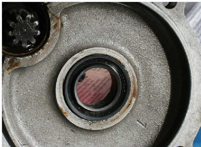
Photo #4 - New lower seal is in place.
