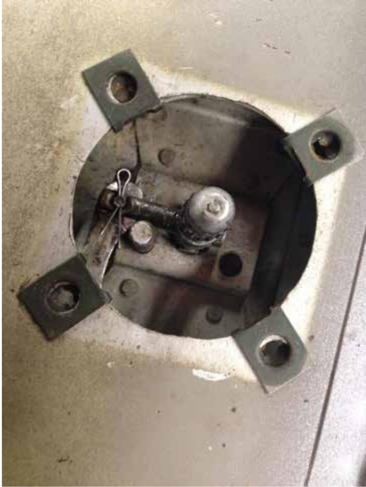
Look inside at the handle shaft and you will see the control arm end that is pinned to the shaft arm with a cotter. In the picture, this is a '48 shaft. Later shafts look different and you may not be able to see the cotter you must remove from the pin to disengage the control arm.
