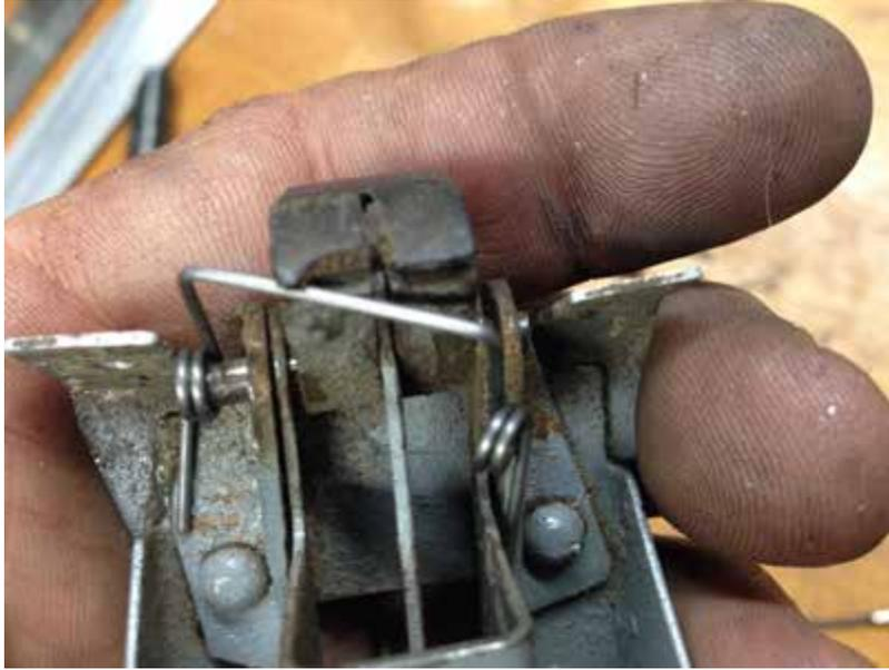
I found it easiest to put the pin back in and get one side of the spring on then push the bar to the other side and get the other side on. The spring rides in the groove of the catch. Needle nose pliers, a pick and patience are your friend here.
