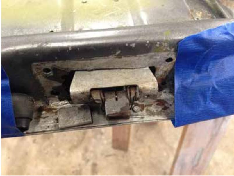
Grab the latch mech., with a pick or needle nose and pull the latch out. Pushing the outside handle helps with this. It will be tight.
