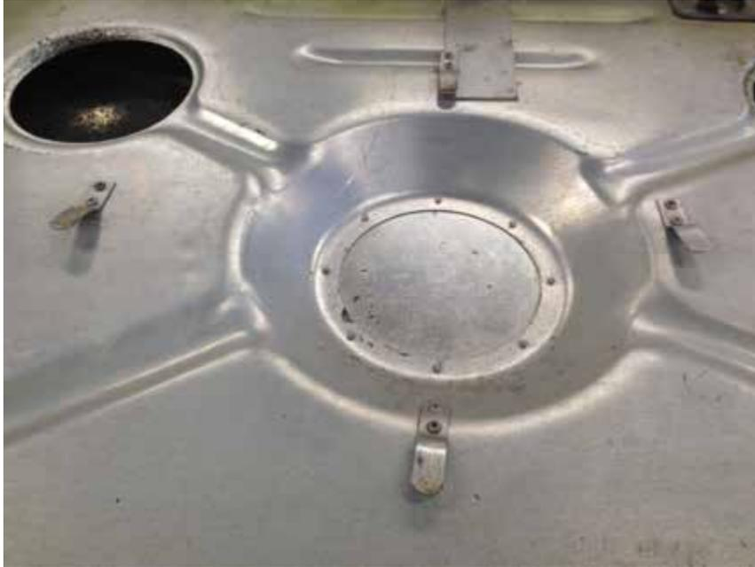
Once you get the front, bottom and aft side detached, if your panel is attached as the original was, you slide the panel down to get it off these brackets.
