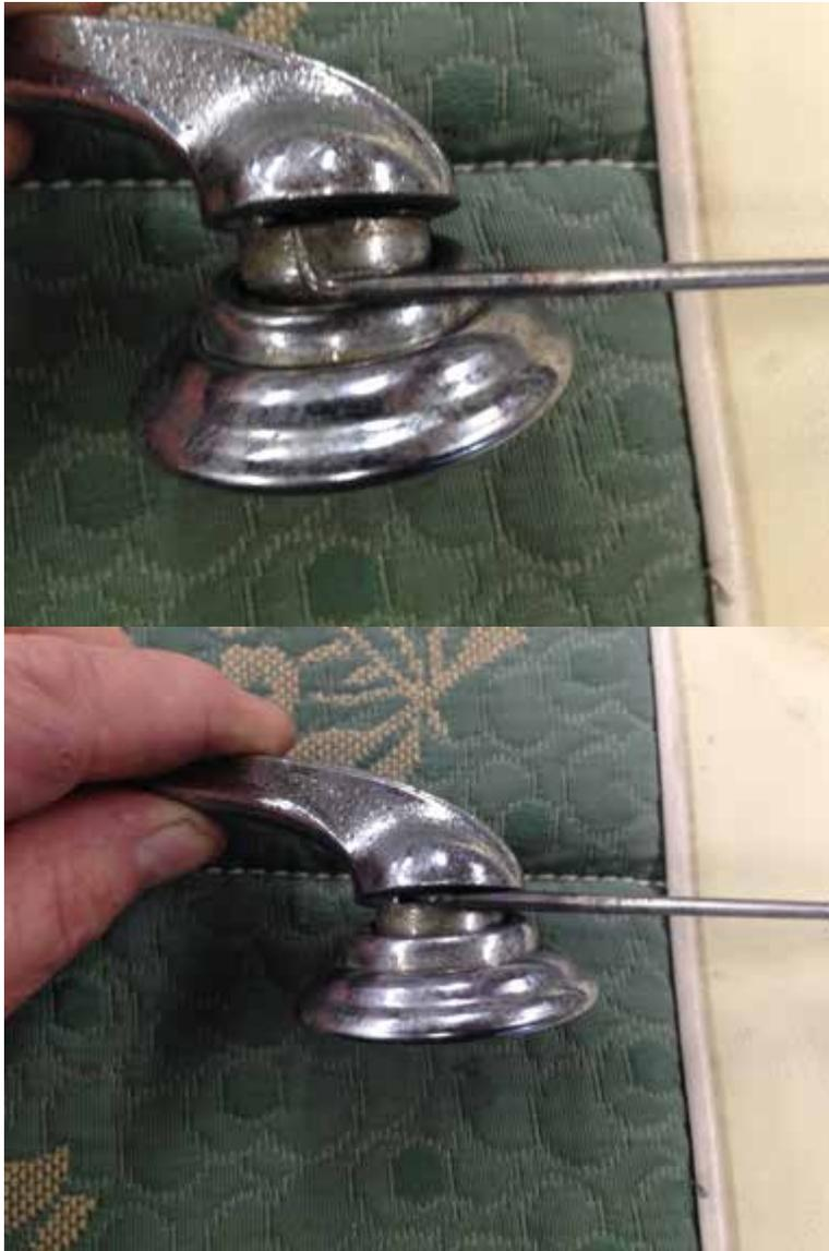
Remove your door handles. From 48 to 53 they were Chevy handles with the U clip you can get out with a pick or the door removal tool for 50-60 era GM cars. 54 and later handles are Ford Mercury and have the same clip and the same tool should work to remove it.
