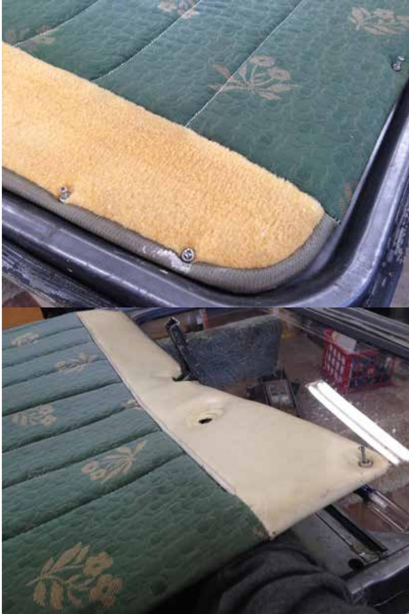
Remove the inside door panel. There may be screws or originally there where just spring clips that you can pry out. Think 50s auto interior.
