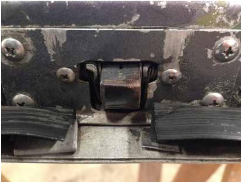
Go to the door jam. Move any weather stripping away to open up an area to remove the latch. Remove the 6 screws you see. If yours is still the original rivets, those will have to be removed and you will want to replace those with screws.
